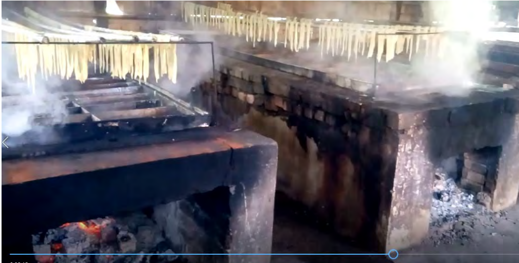
Figure 2.1. Conventional heating using fire wood furnace
