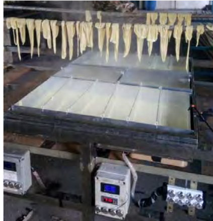
Figure 4.4. Test run of the fabricated induction heating system for fucuk food processing industry
